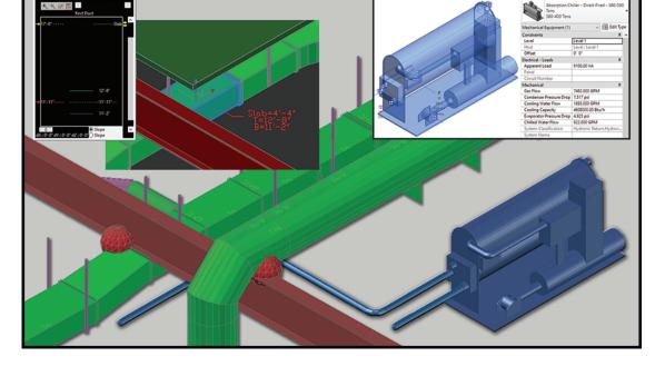
Handling of any drawing entities, both PractiCAD's own and/or 3rd party AutoCAD-based models, preset or user-constructed, is very flexible: you can add grip points to any existing entity, and then save and reuse it as your own. And all 3D entities can be catalogued, too. This simple feature opens up the ability to use any manufacturer's or contractor's equipment or special items very efficiently.
